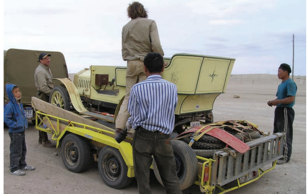
The De Dion doesn't have wheel bearings. It has brass bushes which means every day the wheels had to come off and the bushes needed to be greased.
