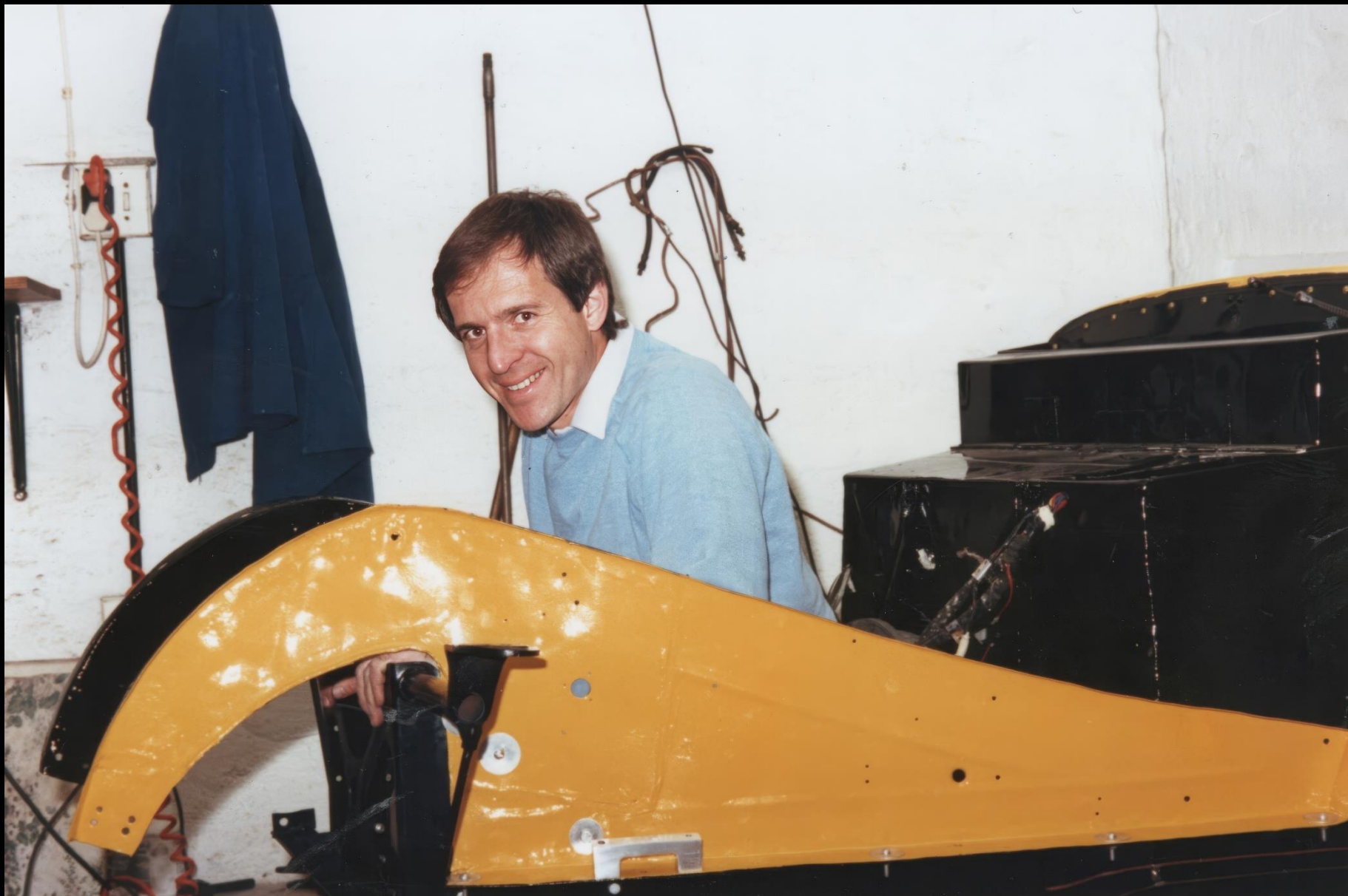
Stan assembling chassis and inner fenders
