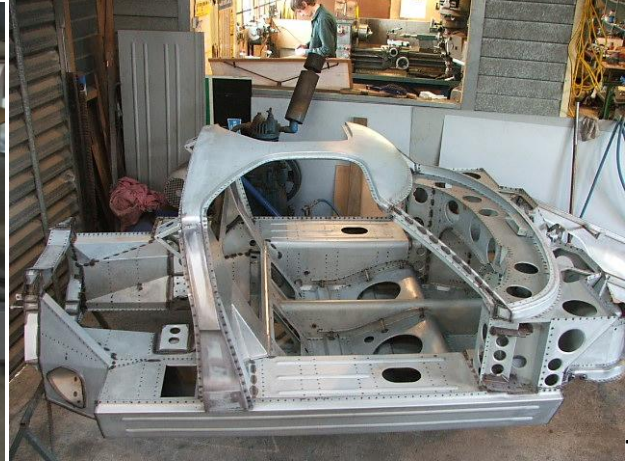
Chassis Construction – so many small parts to make
