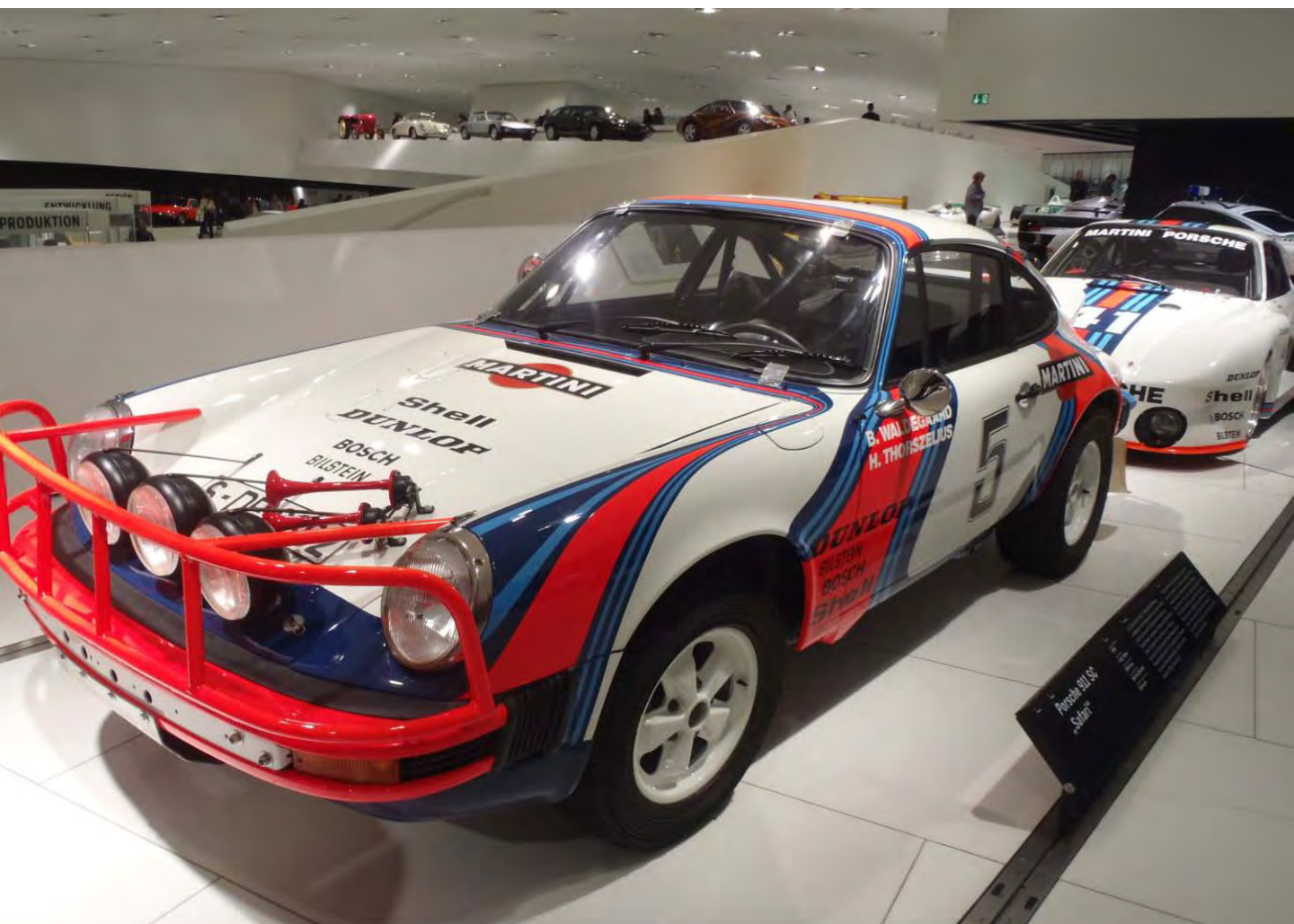
911 in rally mode, with SC Safari, with 11 inches of ground clearance
