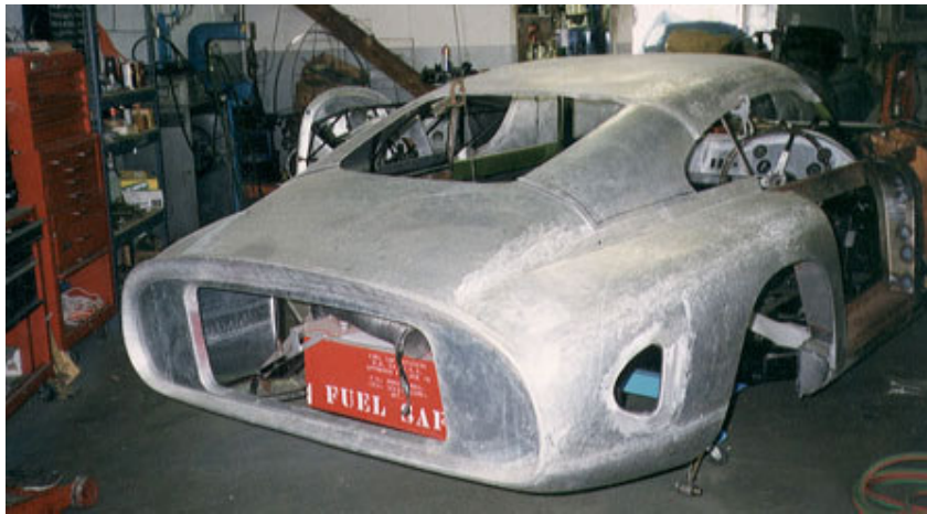
The Kamm tail design on the DP215
